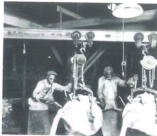
Pouring molten metal into casting molds at National Malleable and Steel Castings, Melrose Park, c. 1945
